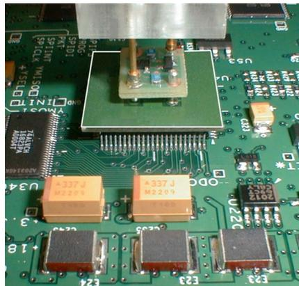
**Figure 3 Sensor Plate Positioned Over an SMT IC**
