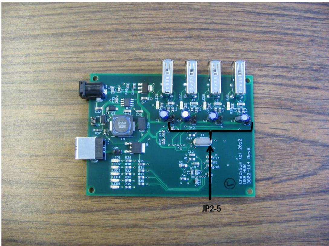
Figure 3. Power distribution jumpers
